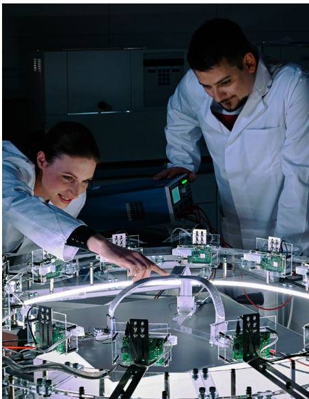
PhD students working together at a multi vision system for deformation measuring of interactive fibre elastomer composites; © ITM/TUD
