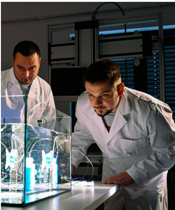
Biomimetic fish fin with dielectric elastomer actuators and fiber reinforcement; © ITM/TUD
