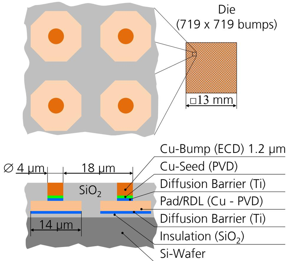
→ Wafer-to-Wafer Bonding (Ø 300 mm) with a 2-step profile (EVG Gemini):
