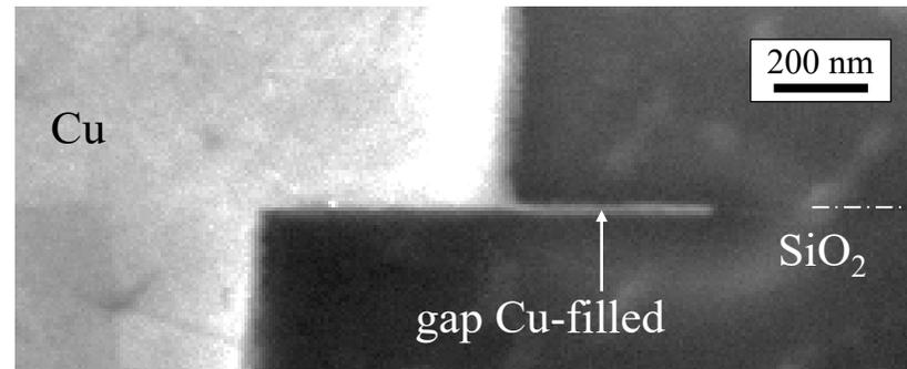
Seamless bonding interface → intergrowth of the Cu grains?
