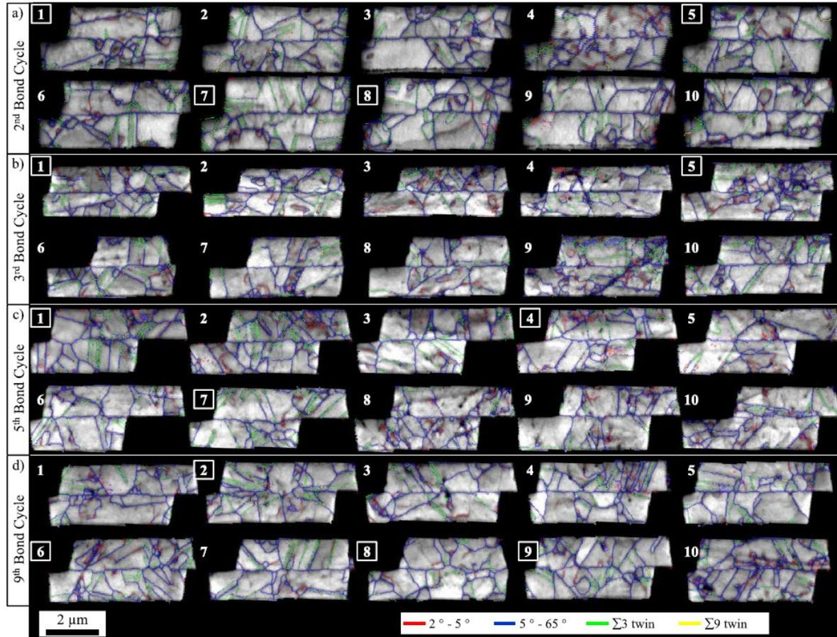
Grain boundary map for all measured interconnects after multiple bonding cycles
