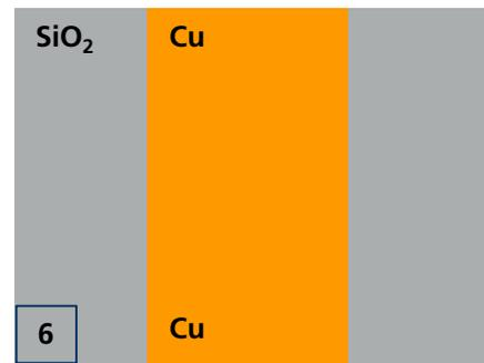
Dies bonded via hybrid bonding
