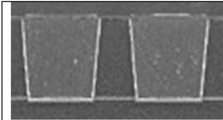
Metal-cross-section of top and bottom metal of transformer have sharp corners!
