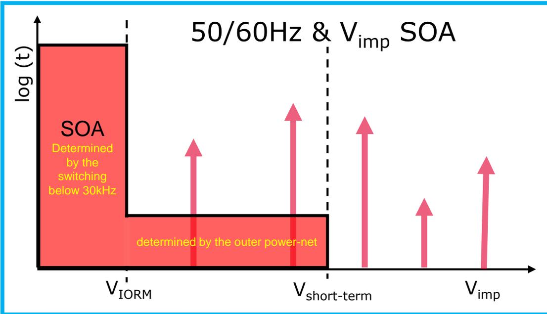
Surge pulses are marked with arrows. The number of surge pulses are not specified in any standard. They can occur at any voltage below  $V_{imp}$ .
