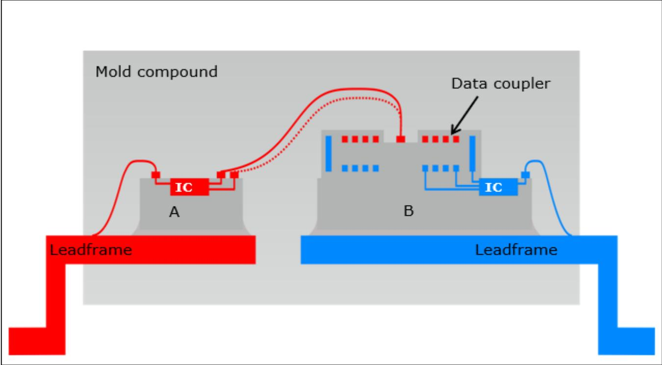
❖ Through a high voltage insulation barrier information and/or energy are transferred.
