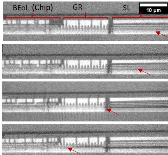
**3D data** during or after micro-DCB test
