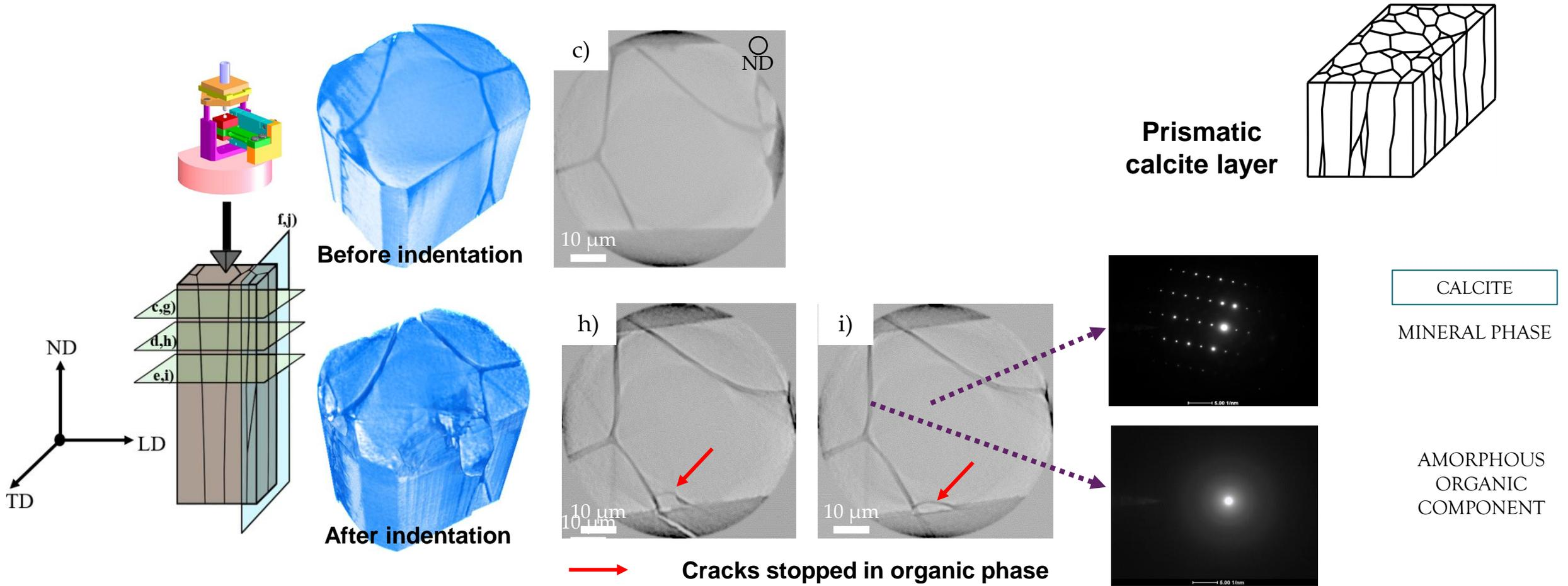
**Cracks formed by indentation propagate in the calcite prism and are stopped in the organic phase**
