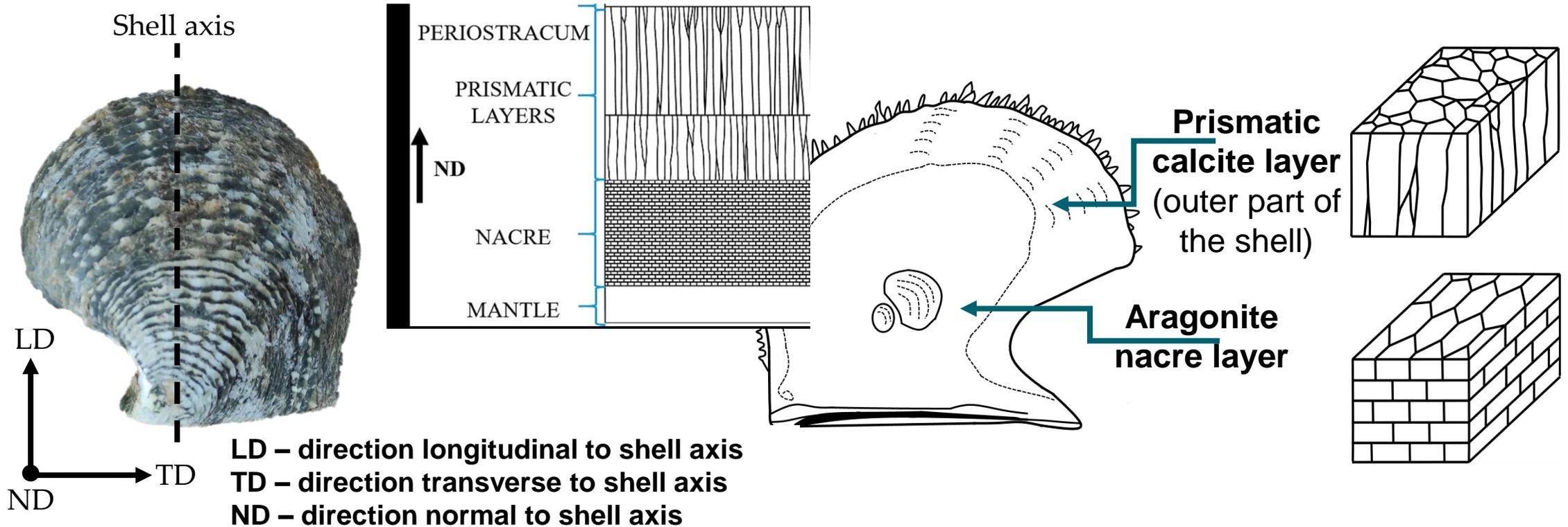
Study of the anisotropy of the mechanical properties of the prismatic columnar calcite layer:
