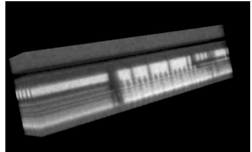
3D data during or after micro-DCB experiment → detailed crack path investigation
