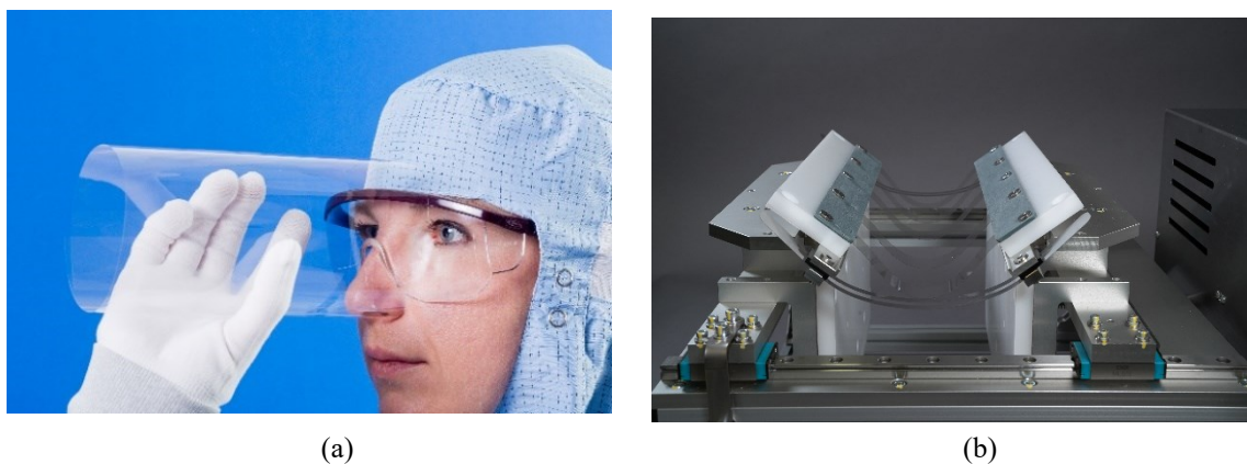
Figure 1. (a) Glass with a thickness below 100 \mu\text{m} is flexible; (b) Early-life fatigue testing of flexible glass
